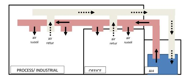
Figure 16.1. Possible Mistake for MVAC Air Distribution for Industrial Office
