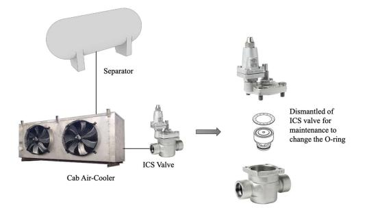
Figure 13.3. Dismantling of ICS Valve for O-ring changes at CAB Air Cooler. (Source: DOSH 2020)
