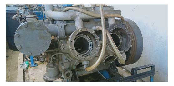
*Figure 13.4.* Abandon compressor pump before the complete maintenance at the factory causing the residual ammonia to release at the opening. (Source: DOSH 2020)
