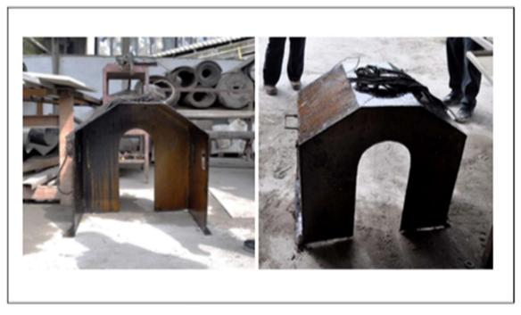
Figure 10.8. Box cover to be installed on the manhole
