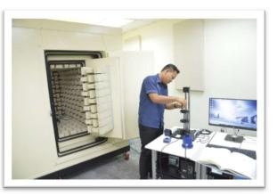
Its main objective is to provide local calibration facility and to produce reliable result for monitoring activities. SECL has been equipped with scientific equipment to calibrate sound level meters, dosimeters and noise calibrators under the standards set by IEC 61672. SECL plans to further expand the scope of calibration to several areas that will include vibration, heat and velocity calibration. It is hoped that the laboratory will be able to
