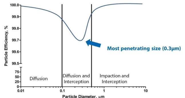
To boost performance in this critical size range, many masks use fibres that have a static charge<sup>[6]</sup>. Disinfecting mask using alcohol removes this charge. **Bottom Line is alcohol deactivates viruses, but it significantly reduces filtration effectiveness.**
