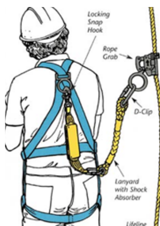
Figure 8: Typical Fall Arrest System
