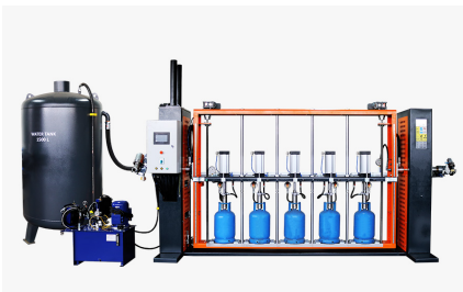
Figure 8: Cylinder Hydrostatic Test Arrangement
